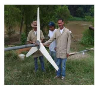
Preparing a Garman type river current turbine rotor for testing.
